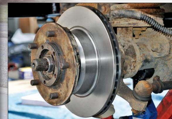
*Top left: Carl slaves away fitting the clutch. Top right: Tom's delicate mechanical skills become evident during wheel bearing changes. Above: Whole new braking system; EBC discs and pads, coupled with Hel braided hoses will take care of stopping.*
