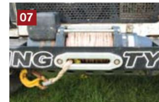
07 Dyneema winch rope. Our Goodwinch 12,000lbs was pretty heavy duty but the main thing was that it gave us peace of mind. This was mounted in front of an Allisport intercooler and two stage Kenlowe fan.
