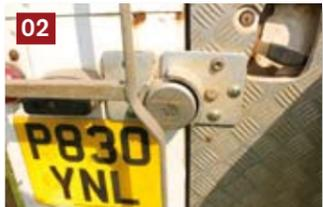
02 Our Kryptonite rear lock is one of the objects that draws the most attention. It's made from steel and can resist prying, cutting and sawing attacks. It really takes a huge weight of your mind knowing the vehicle is secure.
