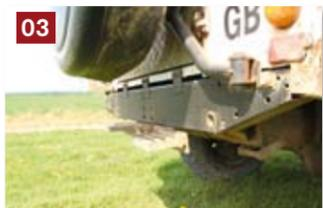
03 We won't forget the day we removed the chequerplate on the rear to find the crossmember crumbled away. We then fitted a new rear Britpart crossmember. The new crossmember allowed us to fit a Paddock swing-away wheel carrier and Dixon Bate recovery assembly.
