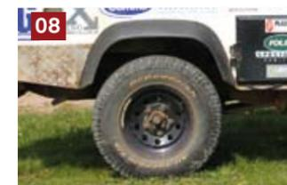
08 Steel modular wheels with standard size BFGoodrich A/Ts from Watling tyres. It is truly unbelievable that we didn't pick up a single puncture.
