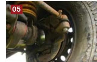
05 EBC vented discs and 4x4 Yellow Stuff brakes. Braided lines by HEL performance. Big Red callipers with new pistons and seals. Polybush expedition mixed kit. Koni shocks, Britpart heavy duty springs. Allmakes wheel bearings and hub swivel rebuild kits. Britpart heavy duty steering arms. D44 Steering guard.
